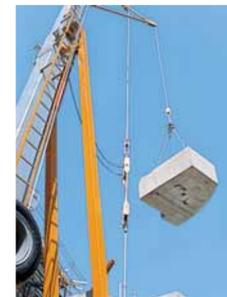
The service derrick allows the ballasts to be positioned without the need for additional means.
